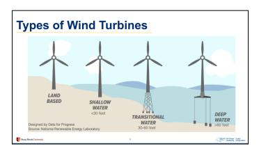
If they are on land or shallow waters, they are fixed foundation turbines. Wind turbines built far offshore or in deeper water are referred to as Offshore Floating Wind Turbines. Over the last decade there has been a push to build wind turbines offshore - far offshore in deep waters.
